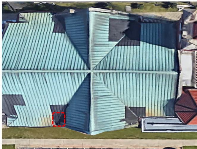
Figure 98. Exterior view of general area shown in Figures 96 and 97 (red dashed outline). Note that roof patches have been completed previously near the location.
